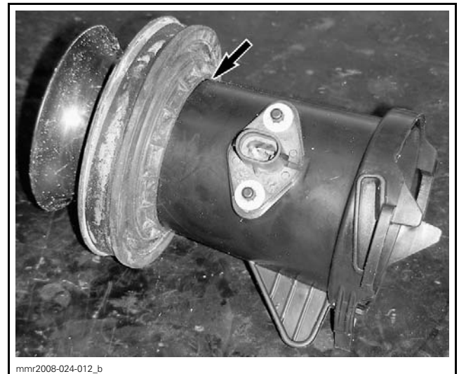
CORRECT BOOT INSTALLATION
